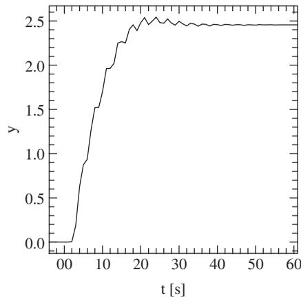
Figure 4. Impulse response of the open-loop system.  $Y = \theta_3$  (rad).
